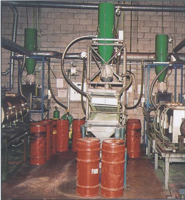
Material is drawn into receiver then discharged into kiln.
