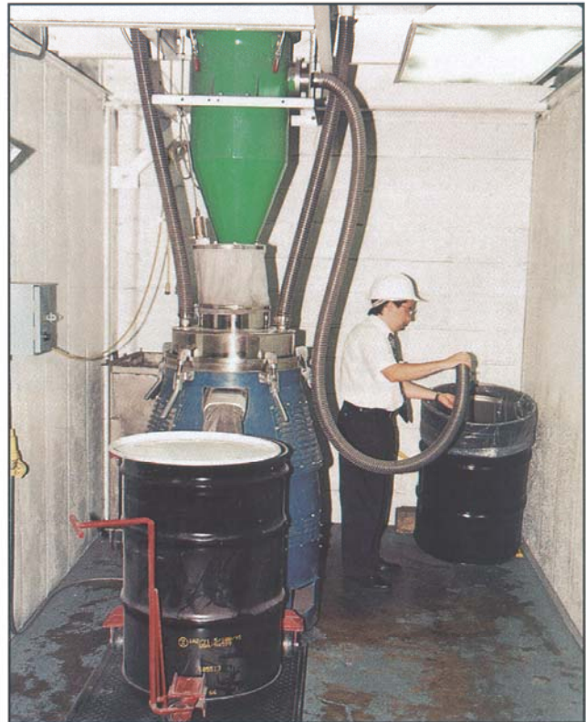
A technician uses vacuum wand to convey material into receiver.
